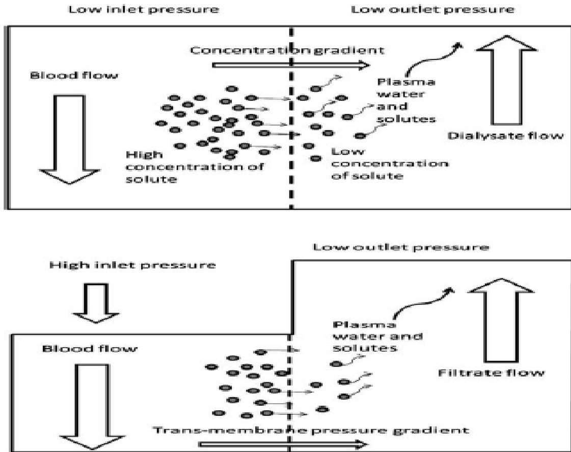
Figure 1 Principles of dialysis (top panel) and filtration (lower panel).
